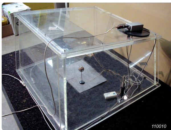
Fig. 32 Measurement in a scale model of a reverberation chamber, using a miniature omnidirectional sound source
