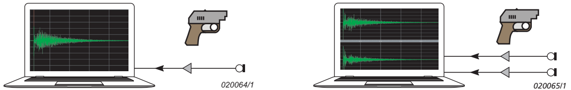
Fig. 17 External Impulse: excitation by impulsive signal, such as from blank pistol or paper bag
