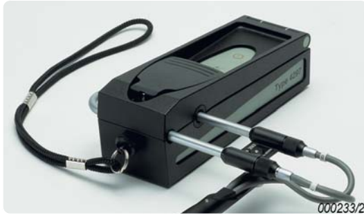
Fig. 9 Complete calibration made using Sound Intensity Calibrator Type 4297
