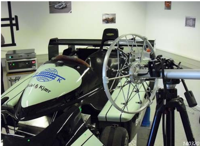
Fig. 2 18-channel sector wheel array positioned on a tripod close to source under test
